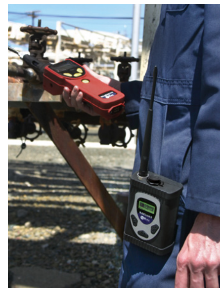
UltraRAE 3000 with RAELink3 used for screening potentially hazardous leaks
